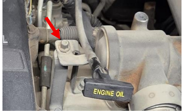
Figure 4: 10MM bolt retaining oil dipstick tube.
