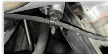
Figure 7B: One of two types of retainers used on harness attached to intake horn. This type is more commonly used in Model Years 2013-2024.
