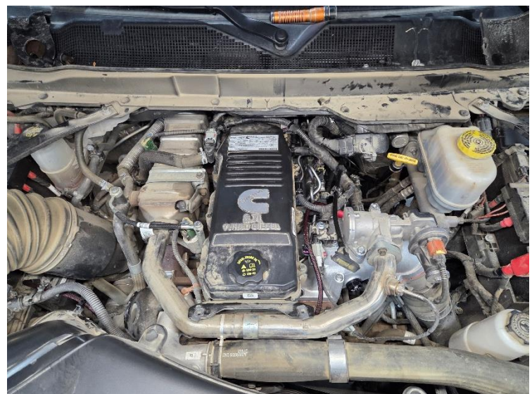
Figure 16: New intake plenum and all necessary components reinstalled.
