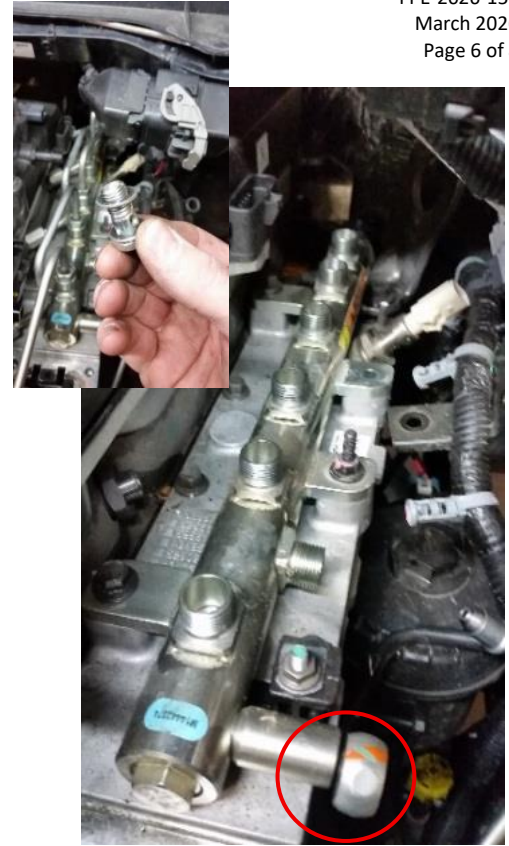
Figure 11: Injection lines removed, fuel return line circled.
