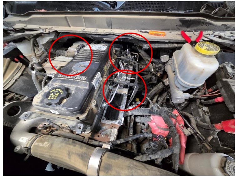
Figure 9: EGR valve, intake horn, and throttle valve removed. PCV and CCV connections circled for clarity.
