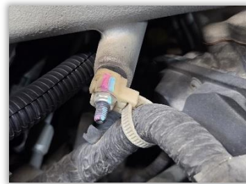
Figure 7A: One of two types of retainers used on harness attached to intake horn. This type is more commonly used in Model Years 2007.5-2012.
